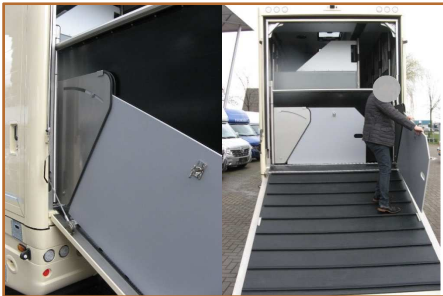
Figure 3.1 Side protections on a horse truck
